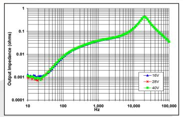
Figure 18: Magnitude of incremental output impedance (Zout = vout/iout) for minimum, nominal, and maximum input voltage at full rated
