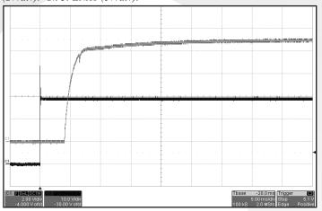
Figure 9: Turn-on transient at full resistive load and zero output capacitance initiated by Vin. ENA1 previously high. Ch 1: Vout (2V/div). Ch 3: Vin (10V/div).
