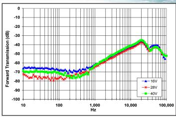
**Figure 19**: Magnitude of incremental forward transmission (FT = vout/vin) for minimum, nominal, and maximum input voltage at full rated
