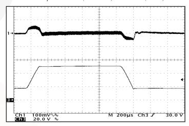
Figure 12: Output voltage response to step-change in input voltage (16V - 50V - 16V) in 150μS. Ch 1: Vout (100mV/div). Ch 3: Vin (20V/div).
