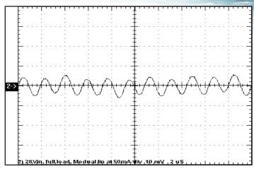
Figure 14: Input terminal current ripple, ic, at full rated output current and nominal input voltage with SynQor MQ filter module (50mA/div).
