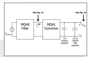
Figure 13: Test set-up diagram showing measurement points for Input Terminal Ripple Current (Figure 14) and Output Voltage Ripple (Figure
