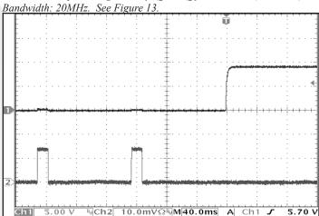
Figure 16: Rise of output voltage after the removal of a short circuit across the output terminals. Ch 1: Vout (5V/div). Ch 2: Iout (5A/div).
