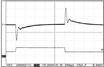
**Figure 10**: Output voltage response to step-change in load current 50%-100%-50% of lout (max). Load cap:  $1\mu$ F ceramic cap and  $10\mu$ F,  $100m\Omega$  ESR tantalum cap. Ch 1: Vout (200mV/div). Ch 2: lout (5A/div).
