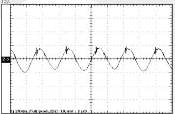
Figure 15: Output voltage ripple, Vout, at nominal input voltage and rated load current (10mV/div). Load capacitance: 1µF ceramic capacitor and 10µF tantalum capacitor. Bandwidth: 10MHz. See Figure 13.
