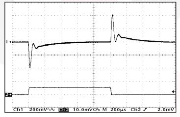
**Figure 11**: Output voltage response to step-change in load current 0%-50%-0% of lout (max). Load cap:  $1\mu F$  ceramic cap and  $10\mu F$ ,  $100m\Omega$  ESR tantalum cap. Ch 1: Vout (200mV/div). Ch 2: lout (5A/div).
